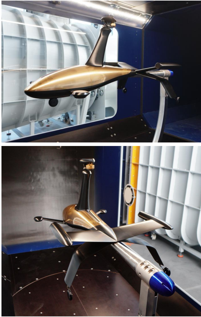
Figure 7. Research object mounted on a mast with a force balance in the wind tunnel.
