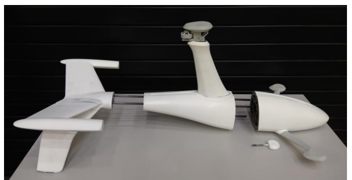
Figure 6. Components of the test object prior to bonding and painting.
