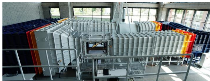
Figure 8. View of the wind tunnel used for research.
