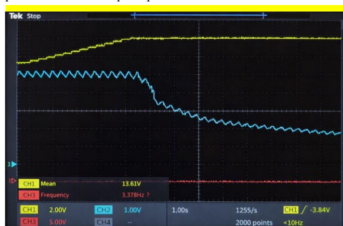
Figure 12. Measured output current and voltage waveforms; total test duration: 13 second.
