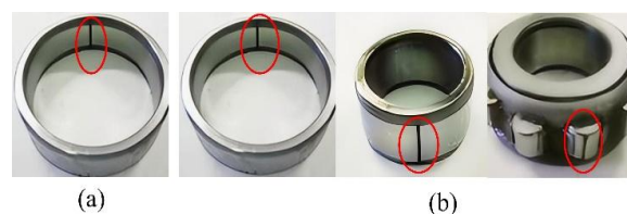
Figure 19. Two kinds of fault bearings: (a) Outer race fault bearing, (b) Comprehensive fault bearing.
