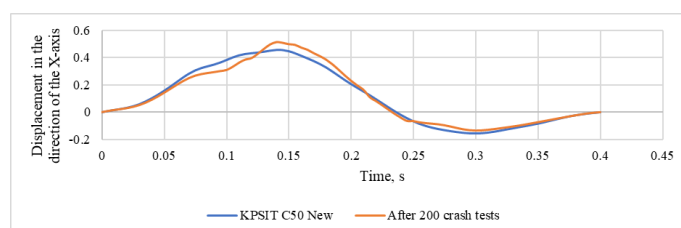
Figure 27. Comparison of the head displacement of the KPSIT C50 dummy towards the X-axis during a frontal collision at 20 km/h for the new state and after 200 crash tests.
