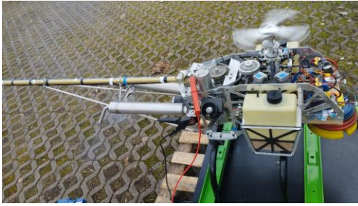
Figure 10. Carrying out measurements of the equivalent sound level L_{Aeq} , the A-weighted level with Slow time weighting L_{AS} , and the 1/3-octave acoustic spectrum for the rotor head without blades – side view.
