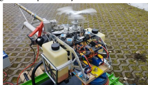
Figure 9. Carrying out measurements of the equivalent sound level L_{Aeq} , the A-weighted level with Slow time weighting L_{AS} , and the 1/3-octave acoustic spectrum for the rotor head without blades.
