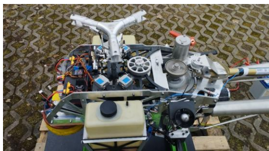
Figure 2. View of the rotor head of the Wabik aircraft with the belt transmission system and the control system.
