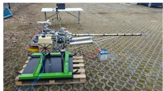
Figure 1. View of the Wabik aircraft with the deployed noise-level measuring apparatus (without rotor).
