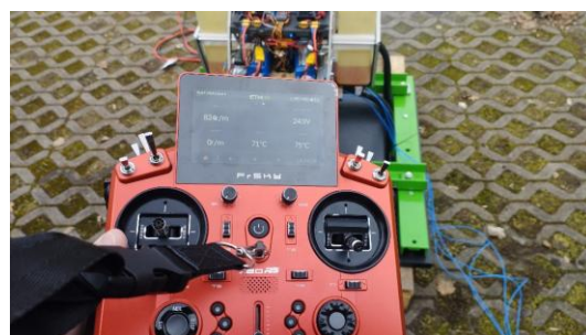
Figure 4. FrSky TANDEM X18SE remote-control system installed in the Wabik aircraft with the possibility of reading head temperatures, supply voltage, and rotor-head rotational speed.
