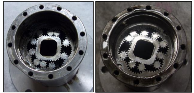
Figure 31. View of the destroyed satellite mechanism. Left: WATER, right: RAPESEED OIL.
