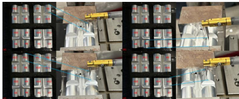
Figure 13. Experimental procedure for roughness reliability evaluation: (a) Group 3, (b) Group 6, (c) Group 11, (d) Group 12.
