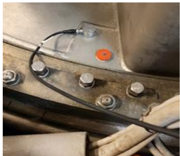
Figure 4. Location of the measurement point: a) schematic, b) actual - installation of the accelerometer on the portside propeller structure of the ship.
