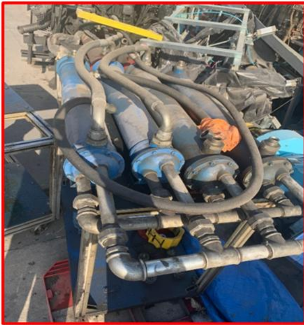
Figure 4. Transition from shell and tube heat exchanger to plate heat exchanger.
