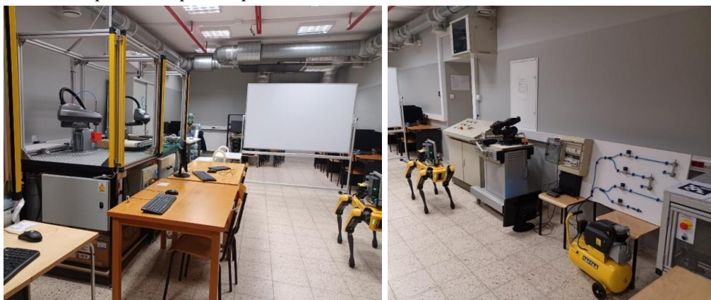
Figure 2. Test environment illustrating a quadruped robot equipped with an inspection system and a malfunction-simulation board.
