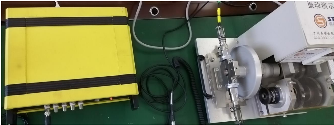
Fig. 3 Rotor test platform.
