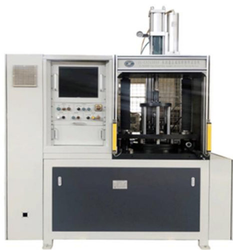
Fig 4. Torsional Characteristic Test Rig for Clutch driven Disc Assembly.
