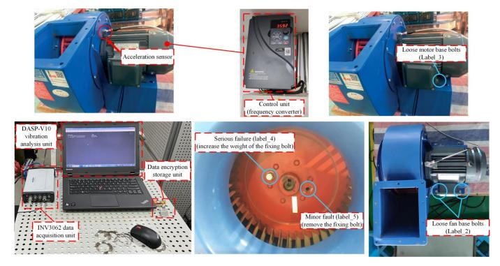
Fig. 6. Auxiliary blower test platform and data acquisition.
