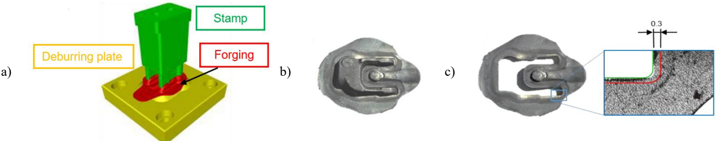
Fig. 2. View of: a) a diagram of the trimming process, b) the forging with flash before trimming, c) the flash after the trimming process in a single-stage setup.
