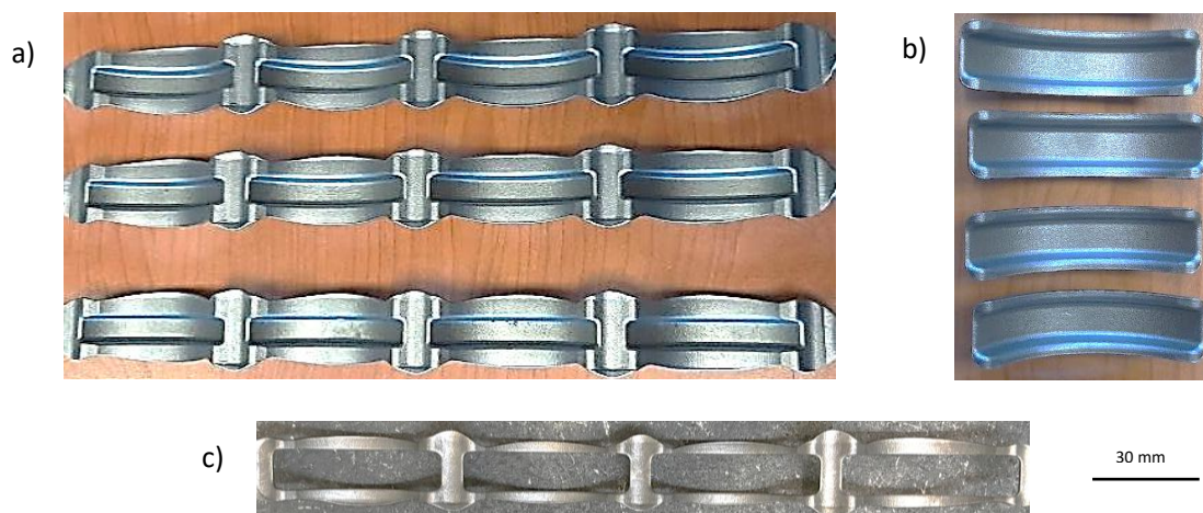
Fig. 6. View of the forging: a) after the four-stage forging process (forgings with flash), b) after flash trimming, c) view of the flash after the trimming process of the four-stage forgings.
