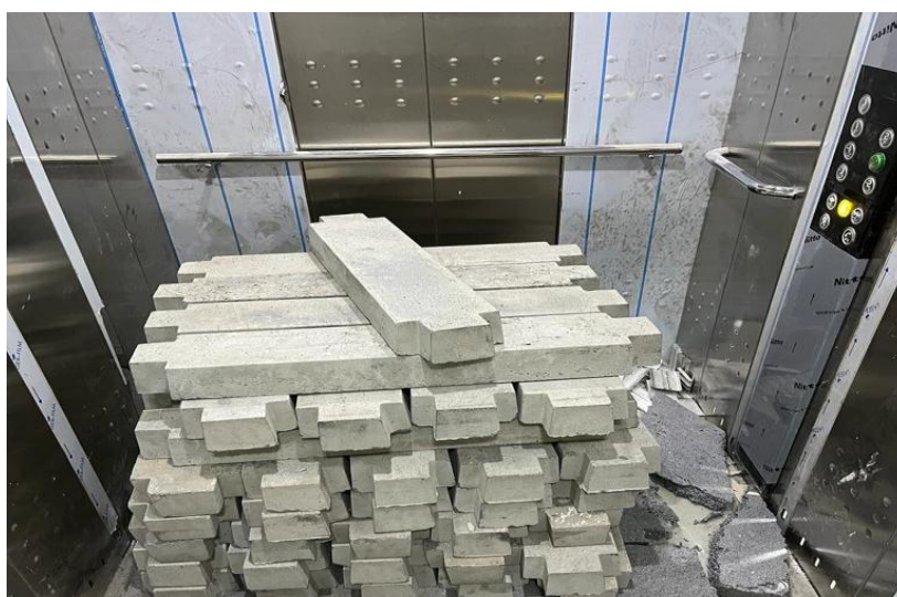
Fig. 9. Homogeneous loading of the cabin with 1000kg weight.
