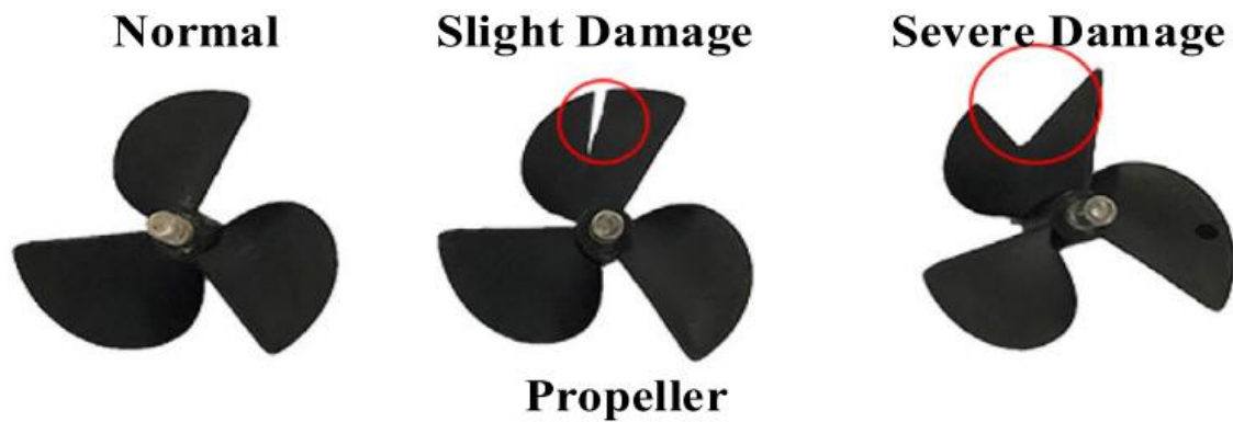
Figure 4. The thruster blade fault type.
