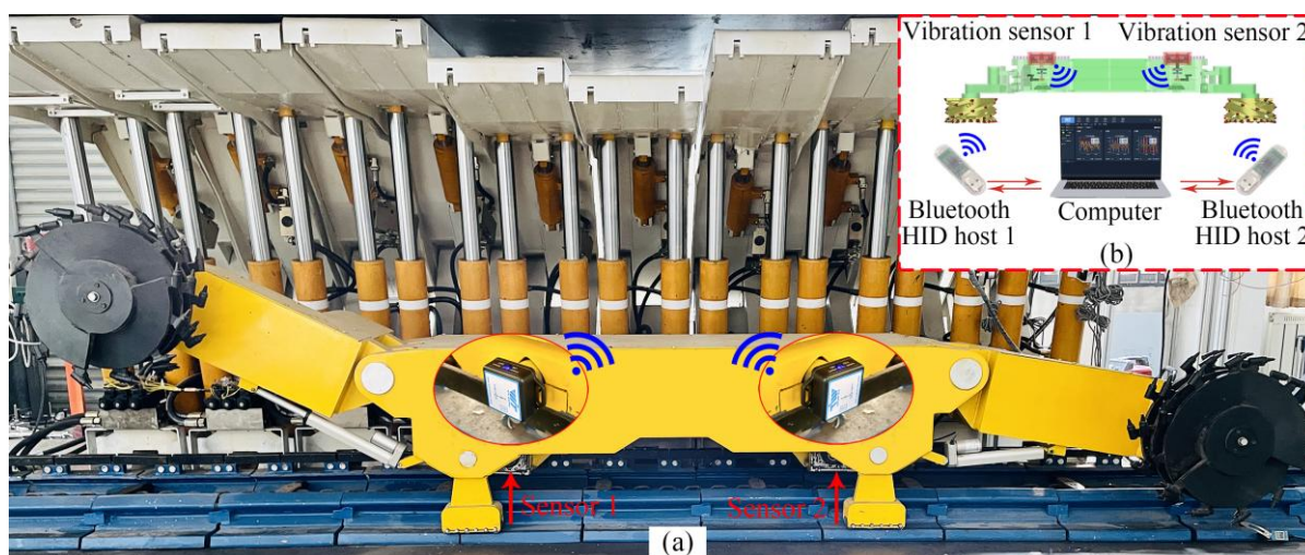
Fig. 6. Shearer traction experiment and its principle: (a) shearer traction experiment system; (b) the experiment principle.
