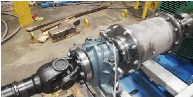
Fig. 5. Innovative flexible clutch mounted at a test rig (in-house resources).
