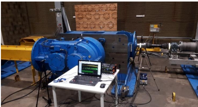
Fig. 6. Drive system subject to tests with the innovative flexible clutch.
