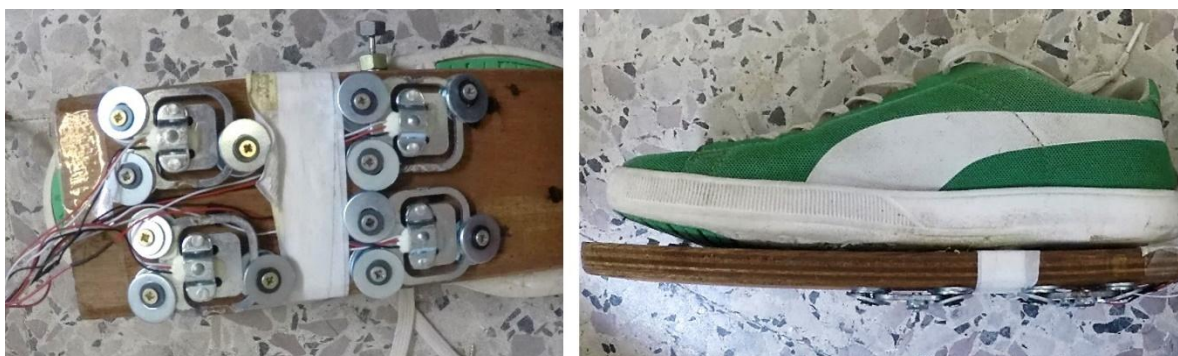
Fig. 2. Views of the right instrumented shoe from below (left figure) and side (right figure).
