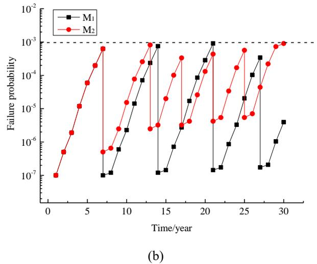
Fig. 8. Comparison of failure probabilities among different maintenances: (a) equal periods maintenance; (b) non-equal periods maintenance.
