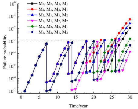
Fig. 9. Changes in pipeline failure probability under different hybrid maintenance methods.
