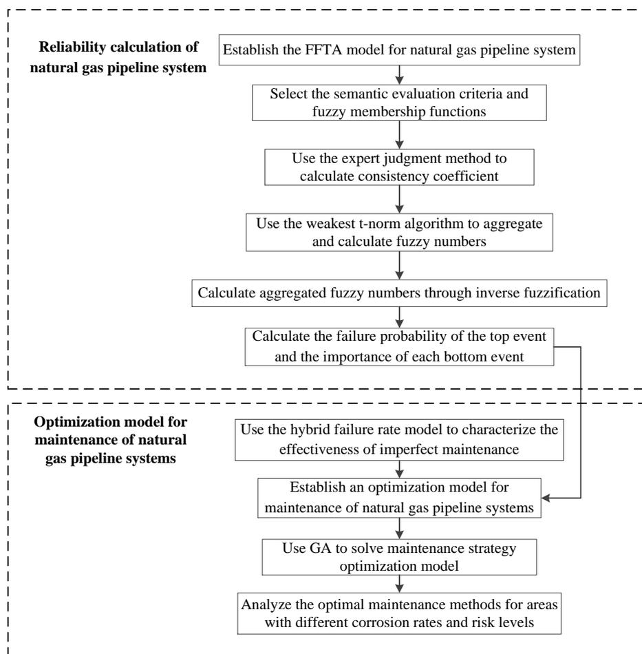
Fig. 1. Optimization process for maintenance of natural gas pipeline system.
