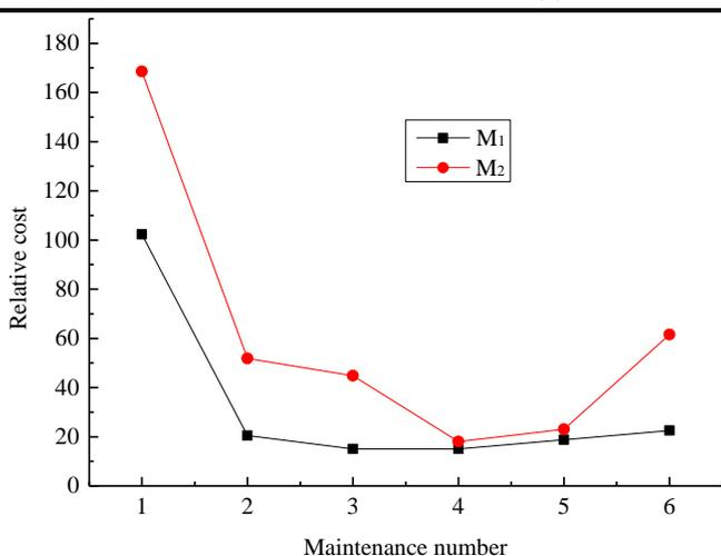
Fig. 6. Changes in relative cost of pipeline systems under different maintenance numbers.
