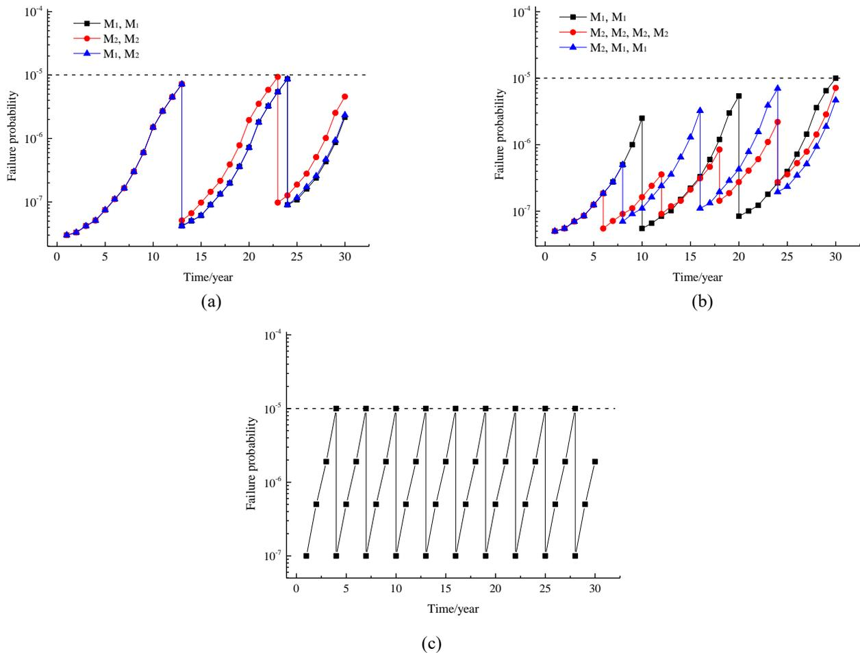
Fig. 13. Changes in pipeline failure probability under different maintenance methods: (a) low corrosion rate; (b) medium corrosion rate; (c) high corrosion rate.
