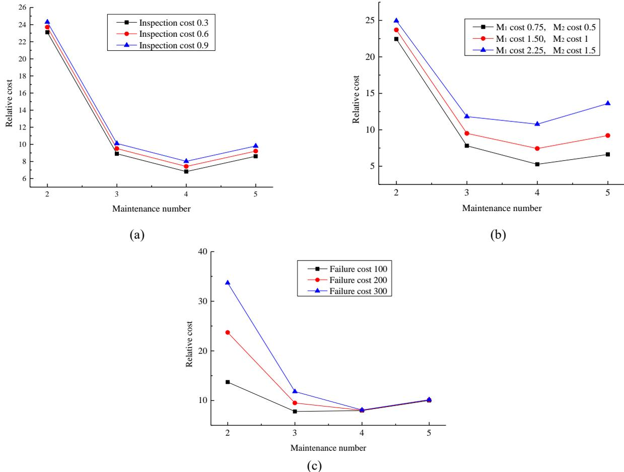
Fig. 14. Sensitivity analysis of maintenance cost parameters: (a) different inspection costs; (b) different maintenance costs; (c) different failure costs.
