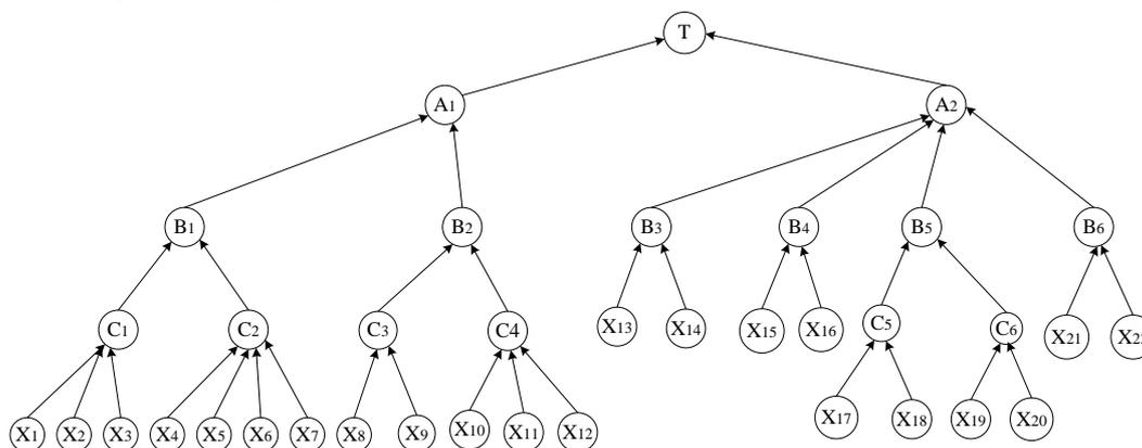
Fig. 3. BN model for natural gas pipeline system.
