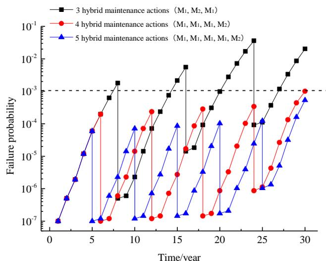
Fig. 7. Change in failure probability of different hybrid
