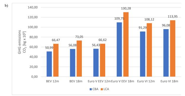
Figure 3. CO<sub>2</sub> emissions from one bus in 2022 a) kg CO<sub>2</sub>/100km, b) in kg CO<sub>2</sub>. Source: authors' own compilation.
