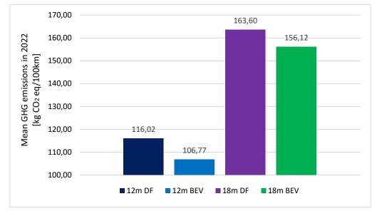
Figure 2. Mean GHG emissions from Euro VI-complaint diesel engine (DF) and electric (BEV) buses for the entire analysed year of 2022. Source: authors' own compilation.
