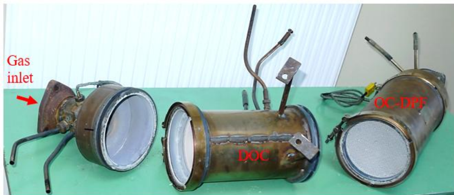
Figure 2. A photograph of the DOC/OC-DPF system with installed exhaust gas intake probes and temperature sensors.
