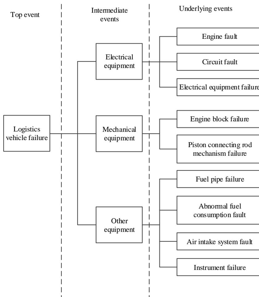
Figure 1. Fault tree structure diagram of logistics vehicles.
