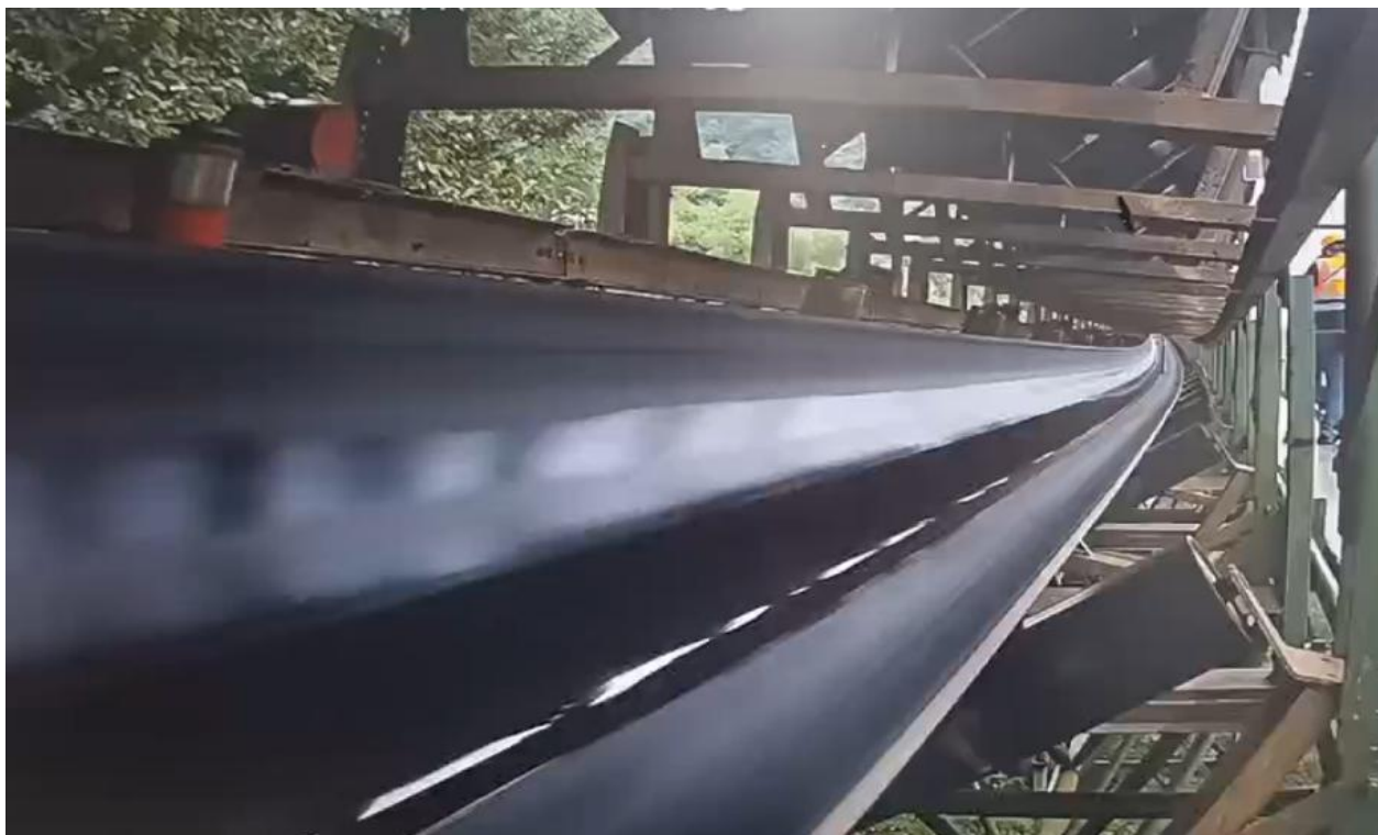
Figure 1. The curve on the tested conveyor.
