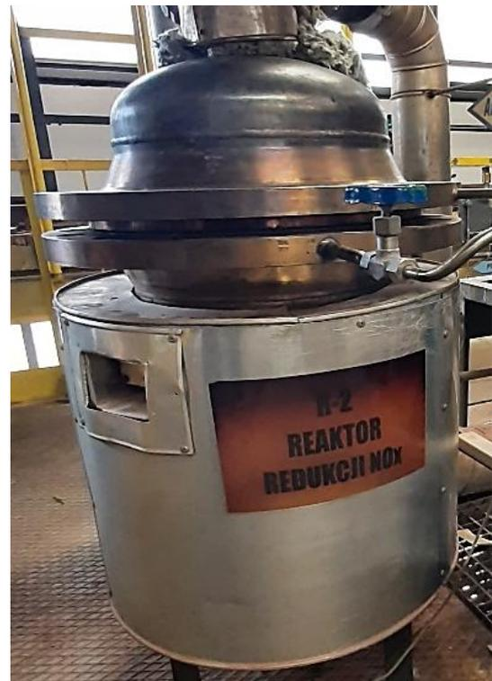
Fig. 1. The SCR-deNO<sub>x</sub>/LT-deN<sub>2</sub>O reactor, constituting one of the technological nodes of the pilot nitric acid plant, on which the geometry of the computational domain was based.
