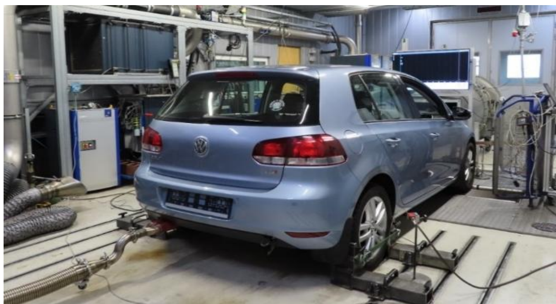
Fig. 3. The references car on the chassis dynamometer during test
