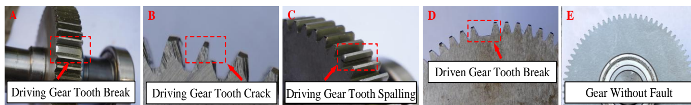
Fig. 6. The real images of different gear failures. C1 is corresponding to A; C2 is corresponding to B; C3 is corresponding to C; C4 is corresponding to A and D; C5 is corresponding to B and D; C6 is corresponding to E without fault.
