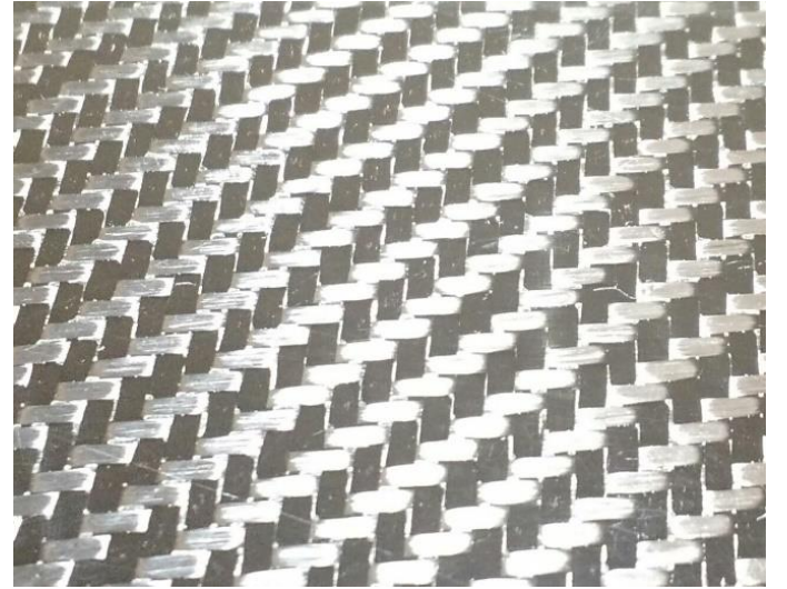
Figure 3. Carbon-fiber composite – structure of the tested material.
