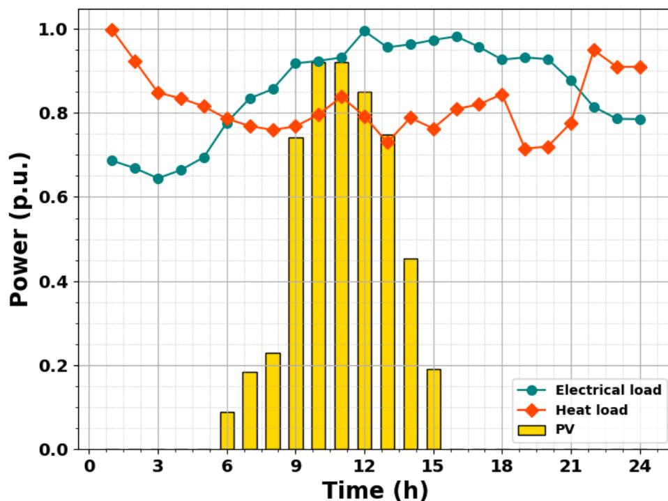
Figure 3. PV Power Generation and Load Projections, Shows estimated 15 MW PV power generation and the peak electrical (176 MW) and thermal loads (53 MW) with distribution across buses.
