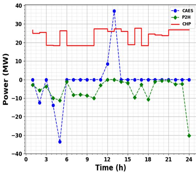
Figure 5. Optimal Thermal Dispatch for the System in the Third Scenario
