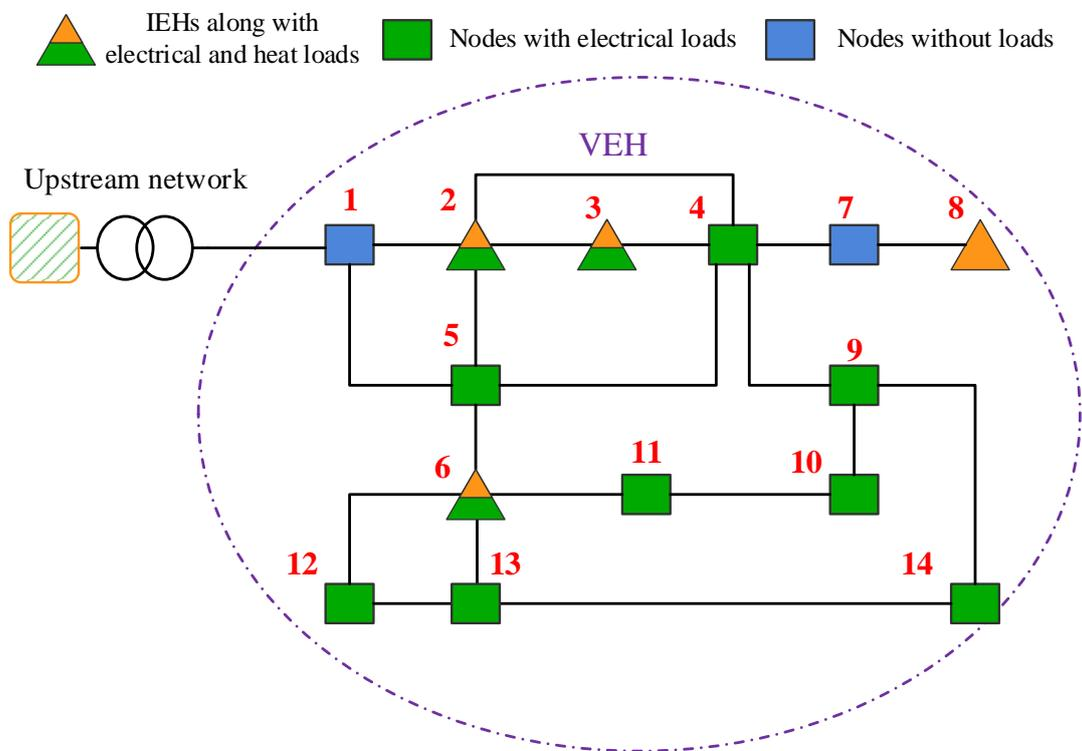
Figure 2. IEEE 14-Bus Test System Configuration.
