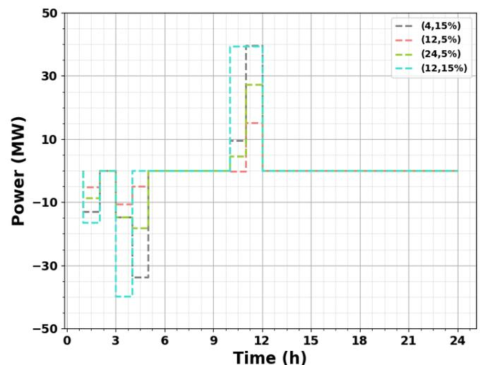
Fig. 8. The sensitivity of compressed air storage planning on robust optimization parameters.
