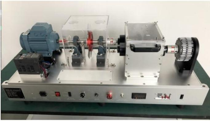
Fig. 8. The bearing test table.
