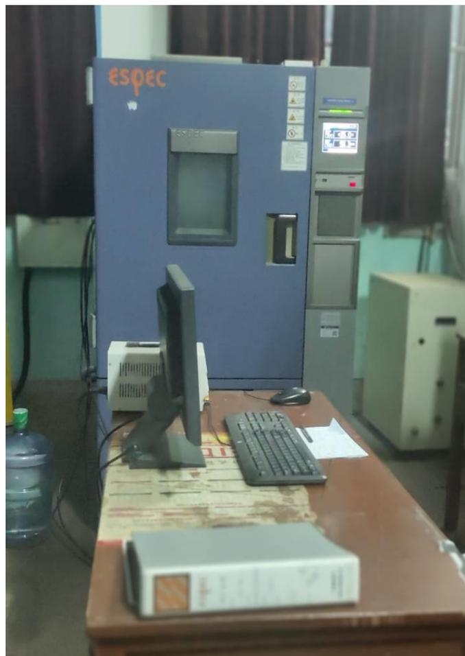
Fig.7. Accelerated life test platform.
