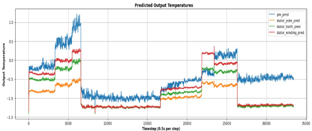
Figure 9. PM, stator\_tooth, stator, yoke and stator\_winding predicted motor output temperature.
