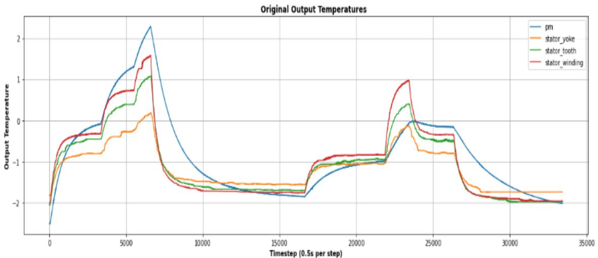
Figure 8. pm, stator\_tooth, stator, yoke and stator\_winding actual motor output temperature.
