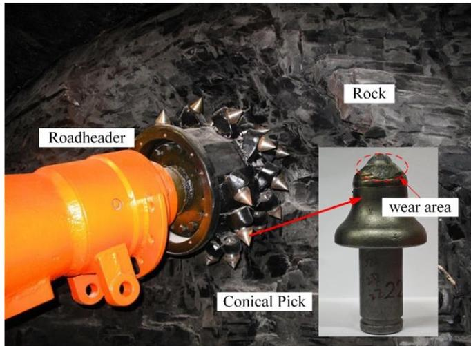
Fig. 1. Wear and tear on roadheader conical picks.
