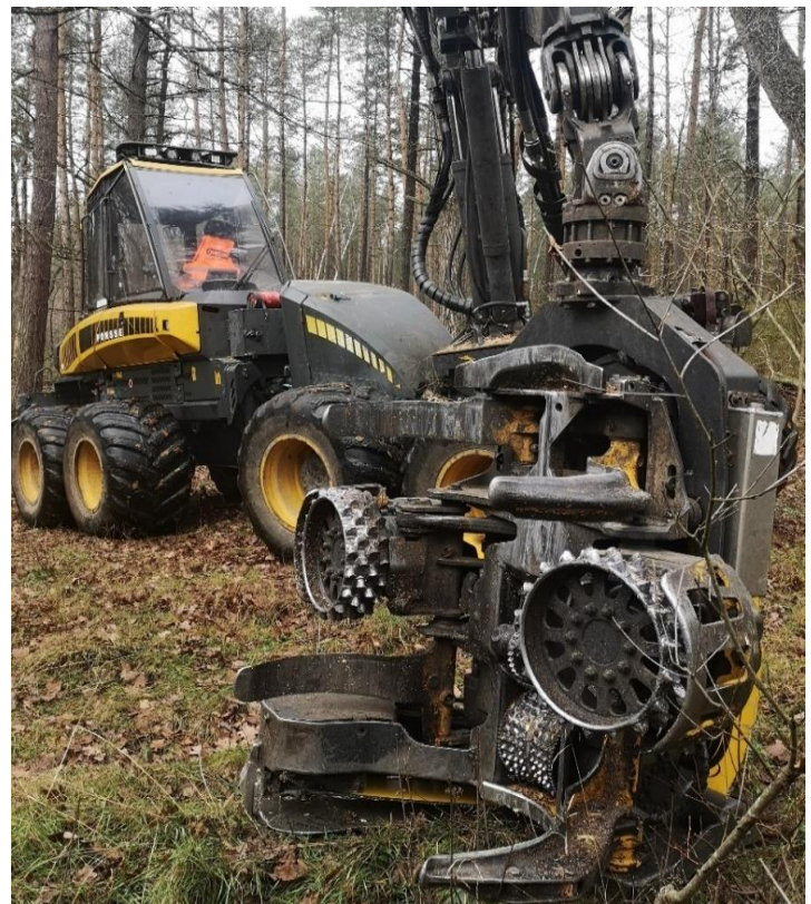
Figure 1. Ponsse Ergo 8W Harvester with an H7 thinning and felling head.
