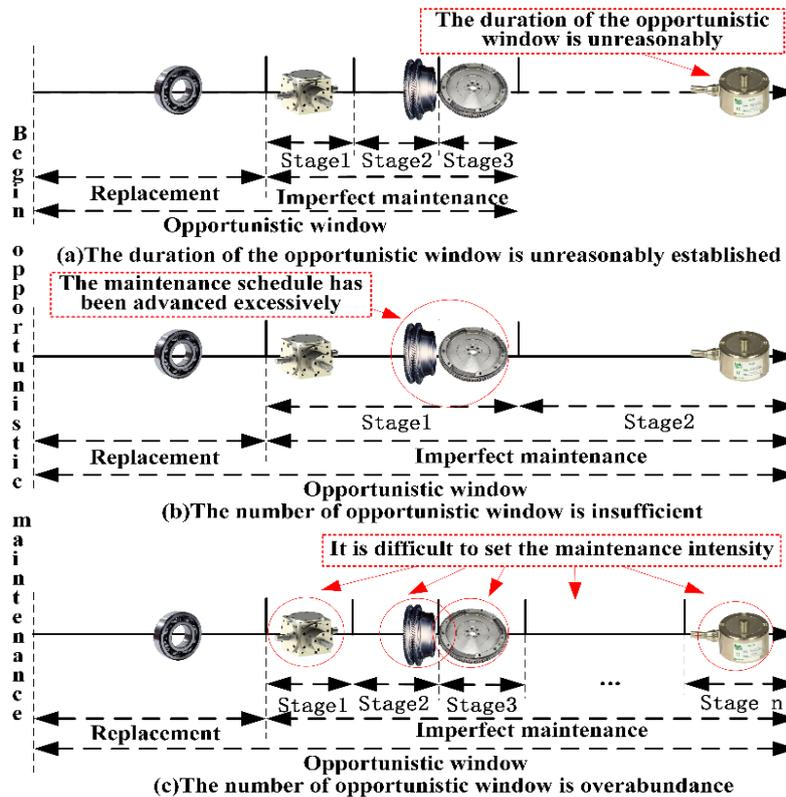
Fig. 1. Schematic diagram of various OM schemes.
