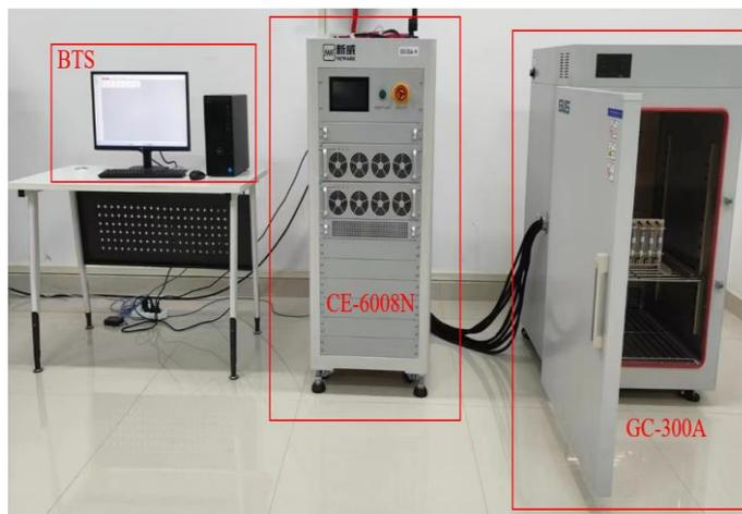
Figure 2. Lithium battery test platform.
