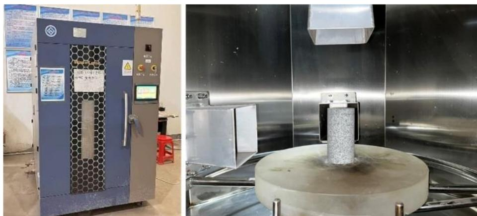
Fig. 3. Exterior and interior view of the Webox-A9 microwave heating system.
