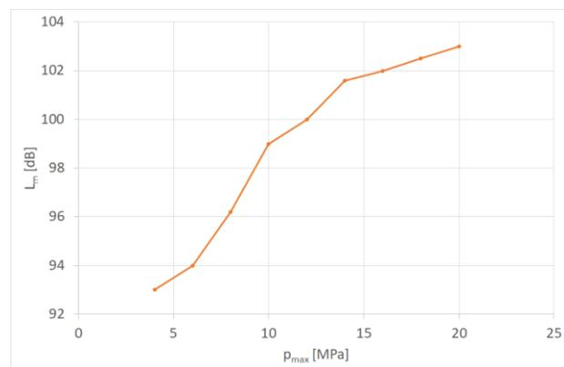
Fig. 6. Dependence of the sound pressure level  $L_m$  [dB] on the maximum pressure value  $p_{max}$  during the start-up of the test system.
