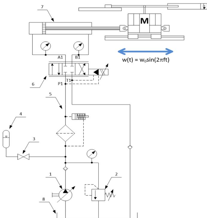
Fig. 3. Diagram of the parts of the hydraulic system of the linear hydrostatic drive simulator: 1 – variable displacement pump; 2 – maximum valve; 3 – shut-off valve; 4 – accumulator; 5 – oil filter; 6 – electrohydraulic amplifier numerous; 7 – setting actuator; 8 - hydraulic oil tank.
