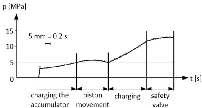
Fig. 4. Actual pressure course during start-up of the test system with the accumulator.
