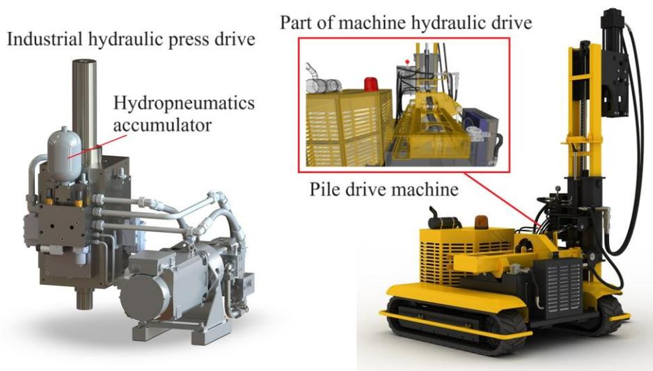
Fig. 1. The example of modern hydraulic drives in mobile machines and industrial systems.
