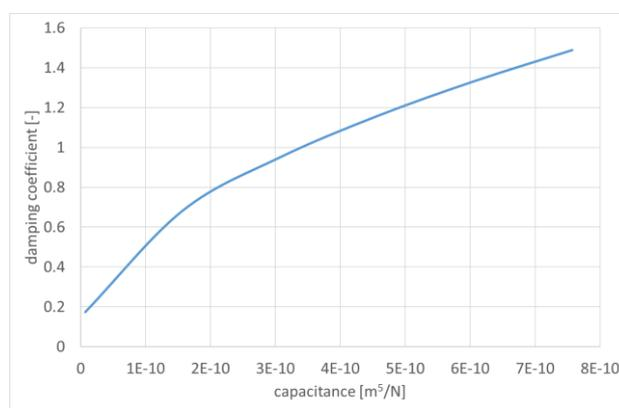
Fig. 5. Dependence of the reduced damping coefficient on the capacitance of the hydrostatic test system (system with the accumulator).
