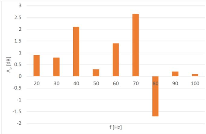
Fig. 8. The ratio of the maximum pressure amplitude for different operating frequencies of the simulator.
