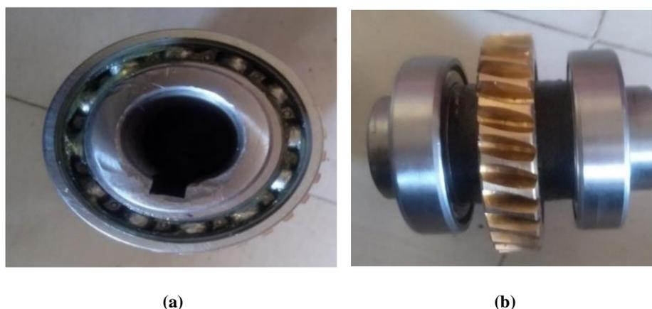
Fig. 3. Good condition (a) worm gear bearing (b) worm gear.
