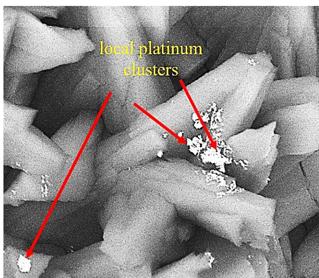
Fig. 3. SEM image of the topography of catalyst surface with 2.5 g/dm 3 Pt content and 20 000x magnification.
