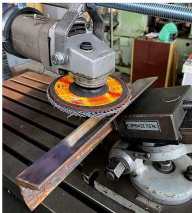
adjust the load of the grinding wheel on the workpiece. The angle change between the working plane of the grinding wheel and the ground plane was carried out by changing the angular setting of the vice. Fig. 7 shows two vise settings: in Fig. 7a, the angle was 20°, and in Fig. 7b, the angle was 2°.
