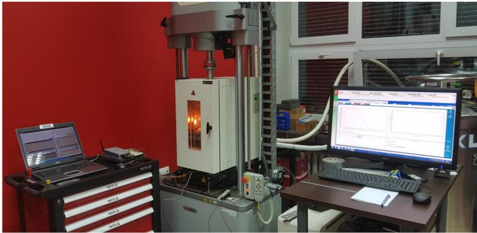
Fig. 1. The test set-up with thermal chamber and excitation system.
