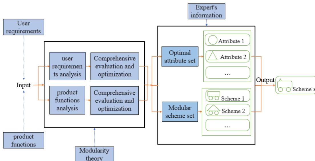
Fig. 5. Early stage of customer-oriented product development process.
