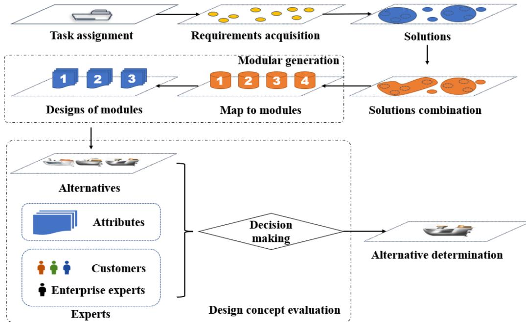
Fig. 1. Process of modular product concept design.
