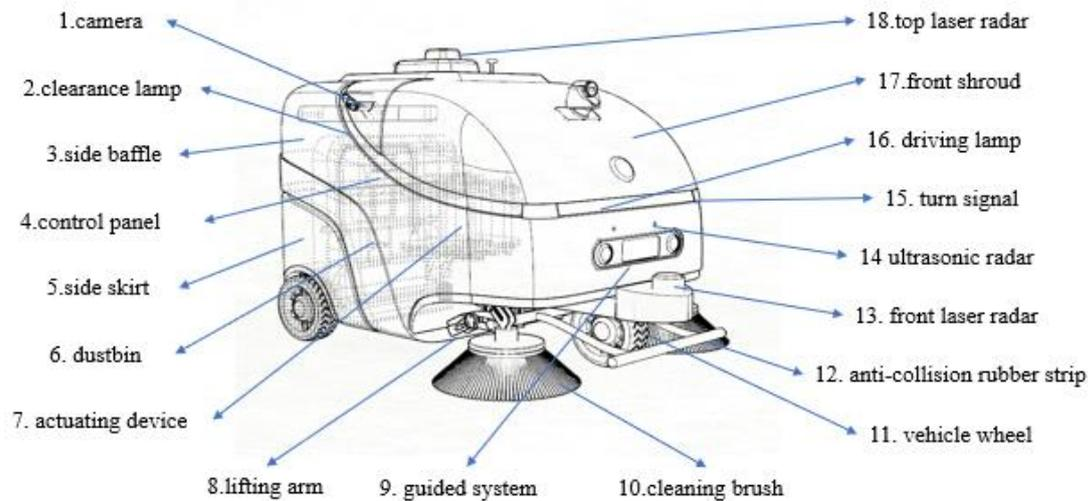
Fig. 6. Components of the intelligent unmanned cleaning vehicle.
