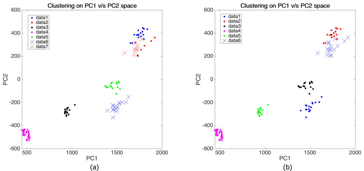
Fig. 9. K-means clustering (a) with 7 classes (b) with 6 classes.
