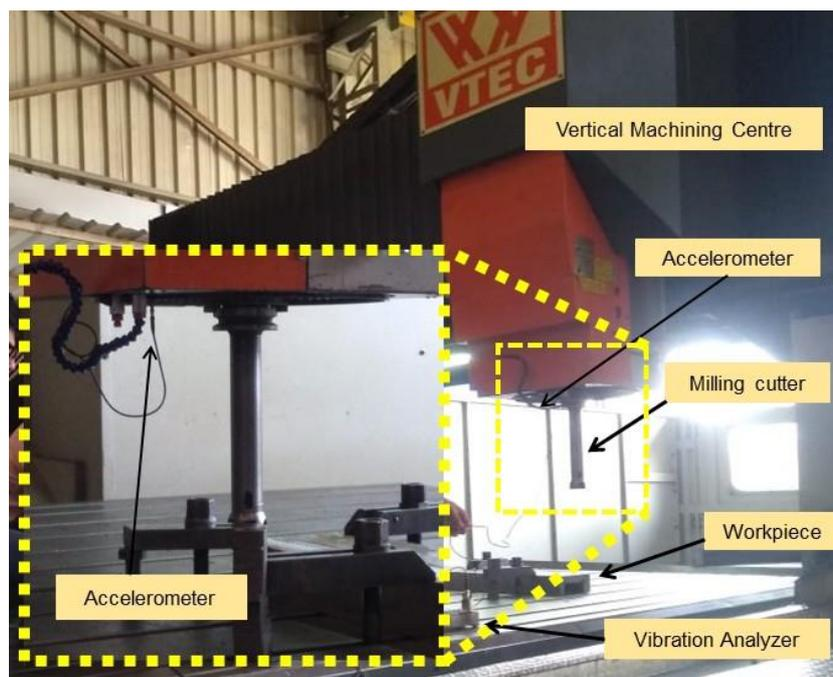
Fig. 1: Experimental Setup.
