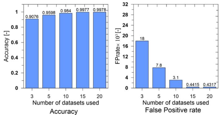
Fig. 12. Sensitivity of methodology to number of datasets used for training a) Accuracy b) False Positive Rate.
