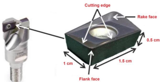
Fig. 3. Defect-free (Normal) insert with the dimensions.
