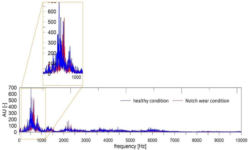
Fig. 7. Comparison of frequency domain signals in different conditions.
