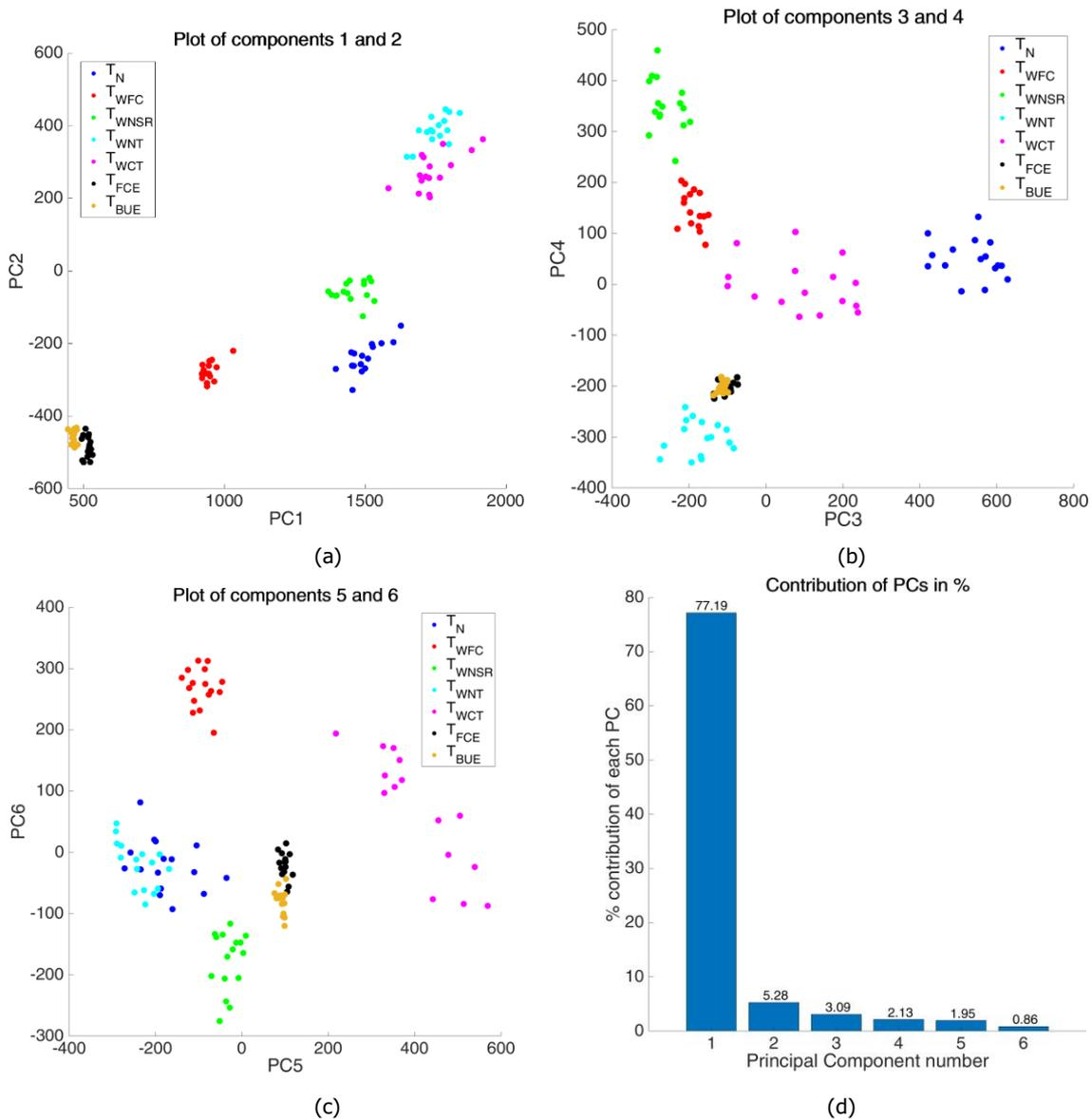
Fig. 8. PCA projections for training data set (a) PC1 v/s PC2 (b) PC3 v/s PC4 (c) PC5 v/s PC6 (d) Contribution of first 6 PCs.
