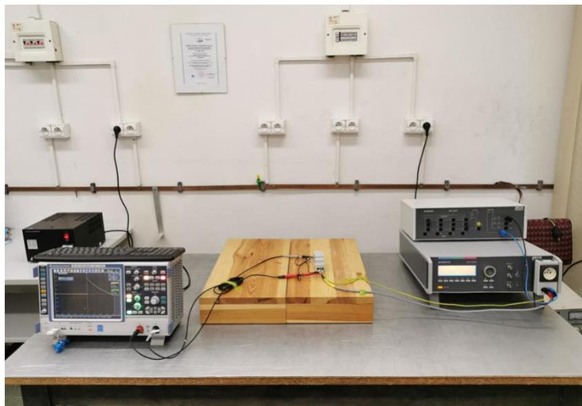
Fig. 10. Test bench for studying electric surge immunity of a PW-2-32 and PW-S surge arrester.
