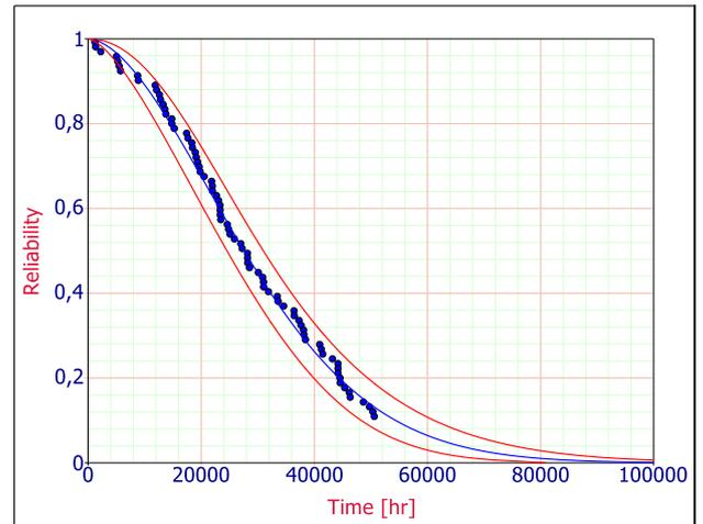
Fig. 5. 2P-Weibull reliability function for the superstructure with the 95% confidence interval.
