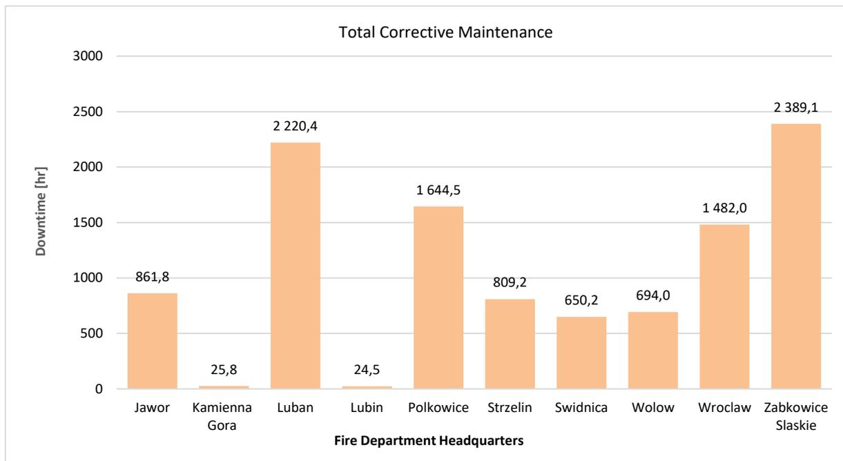
Fig. 14. Total corrective maintenance downtime for the chassis/cabin and the superstructure.
