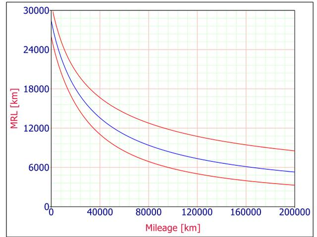
Fig. 10. *MRL* for the chassis/cabin with the CI 95%.
