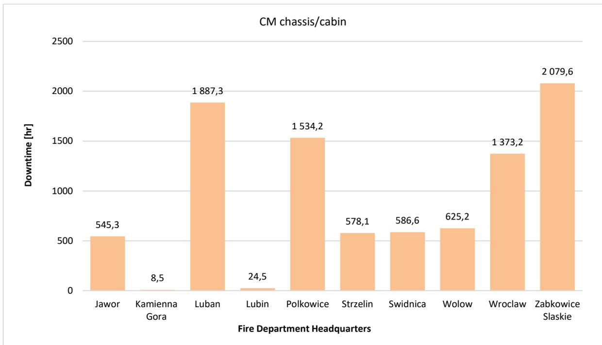
Fig. 12. Corrective maintenance downtime for the chassis/cabin.
