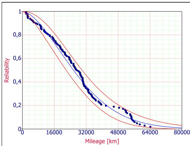
Fig. 4. 2P-Weibull reliability function for the chassis/cabin with the 95% confidence interval.
