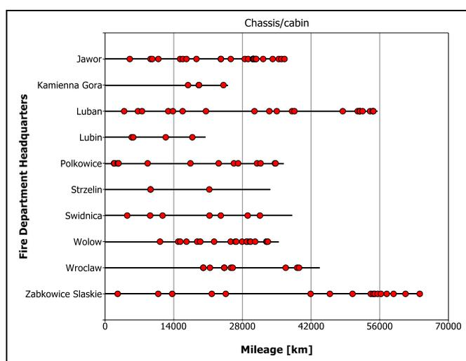
Fig. 2. System operation for the chassis/cabin – exact failure time in kilometres.
