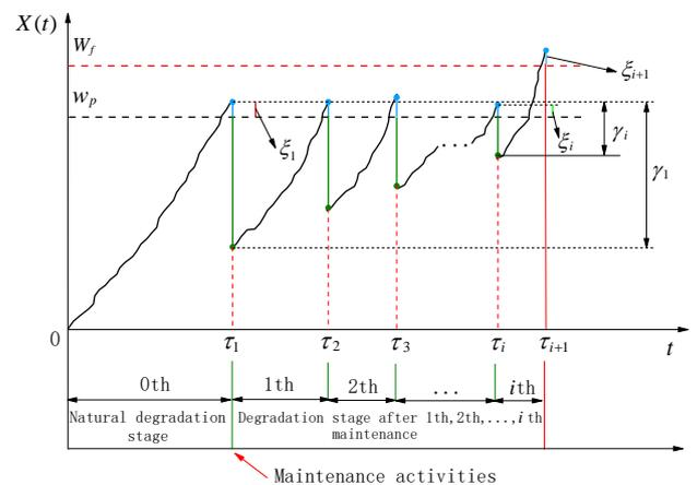
Fig. 1. Equipment degradation track under the influence of maintenance.
