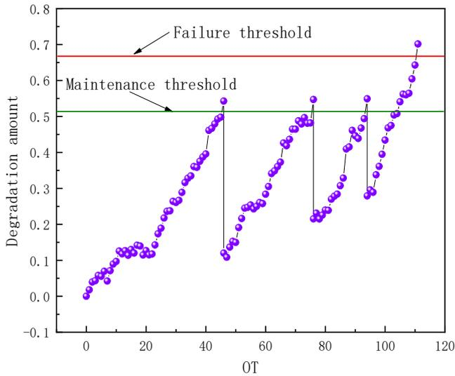
Fig.2. Simulated degradation data under maintenance influence.
