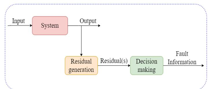
Fig. 1. Fault Diagnosis using data driven approach.
