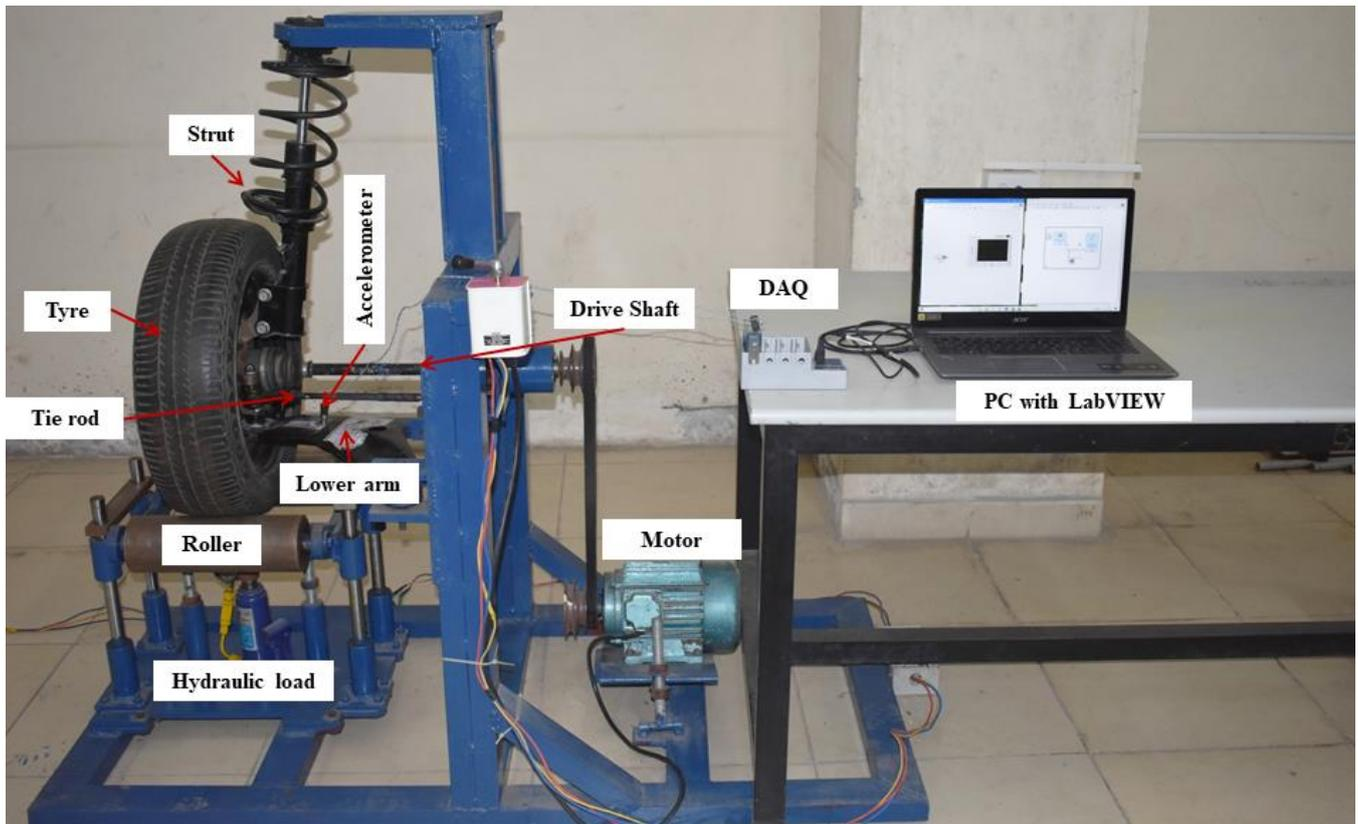
Fig. 3. Experimental setup of suspension system.
