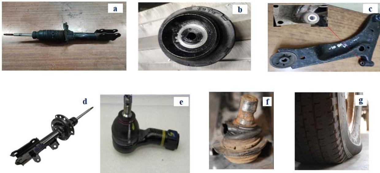
Fig. 4. Faults in the McPherson suspension system
