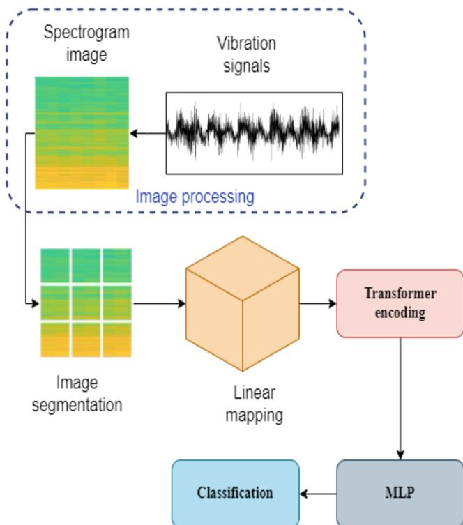
Fig. 2. Work flow of fault diagnosis of suspension system using vision transformer.
