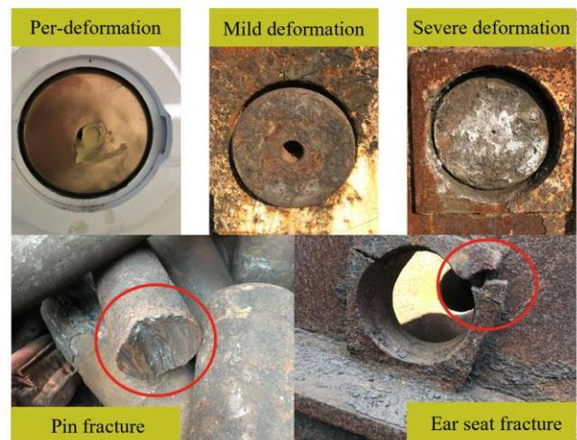
Fig. 1. pin connection of hydraulic support.
