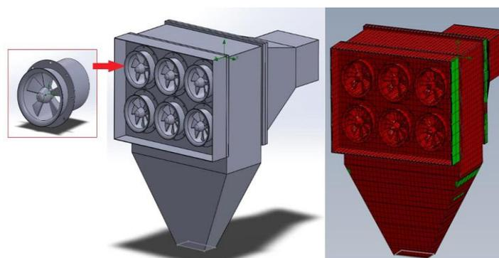
Figure 10. MOS type multi-cyclone, consisting of 6 cells with a blade pitch angle of 45° and a simulation mesh of the object.
