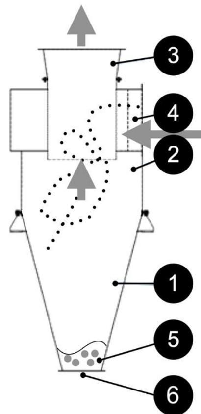
Figure 1. View of the internal structures of a dry centrifugal dust collector (own work inspired by [36]); 1 – chute, 2 – cylindrical cover, 3 – gas outlet pipe, 4 – inlet port, 5 – dust captured, 6 – dust removal nozzle, dotted spline: dusted air spin.
