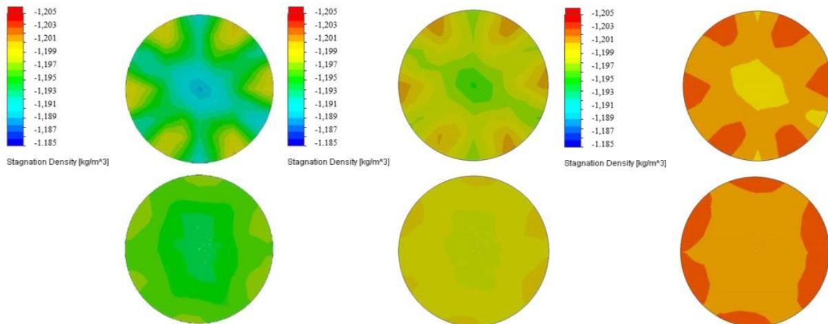
Figure 14. Longitudinal section of a MOS cell (cyclones No. 1 in the left figure, No. 2 in the centered figure, No. 3 in the right figure), equipped with 6 blades, inclined at an angle of 45° showing the distribution of the density of the air, behind the blades, polluted with lignite dust (top row picture) and at the outlet (bottom row picture) at a volumetric flow of 0.4 m<sup>3</sup>/s (left figure), 0.3 m<sup>3</sup>/s (centered figure) and 0.2 m<sup>3</sup>/s (right figure).
