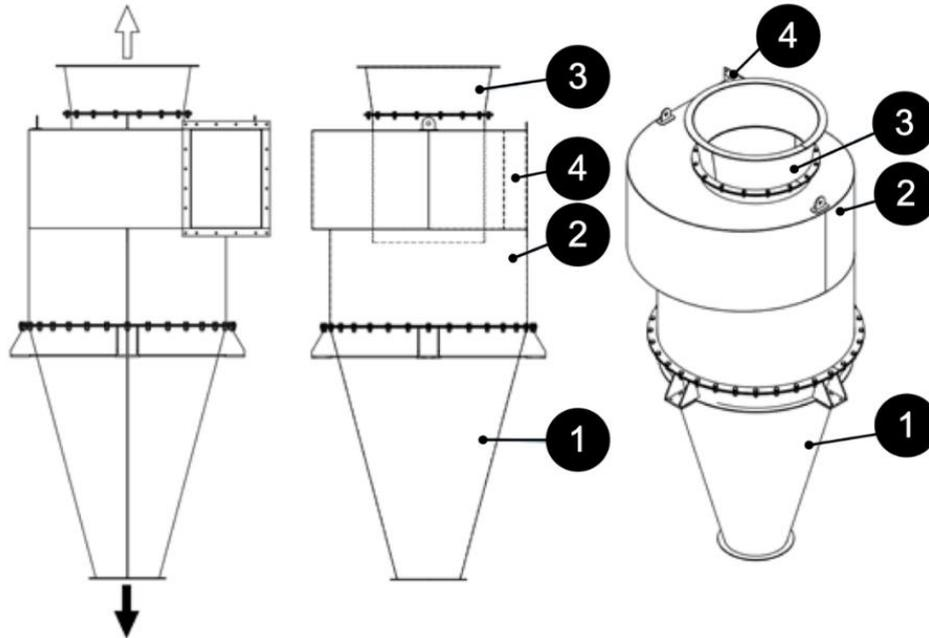
Figure 2. Views of the design of a dry centrifugal dust collector: 1 – dust chute, 2 – cylindrical part of the cyclone (cylindrical cover), 3 – diffuser and gas outlet (gas outlet pipe), 4 – inlet port (illustration borrowed and reproduced with the permission of the Instal-Filter S.A. entrepreneurship).
