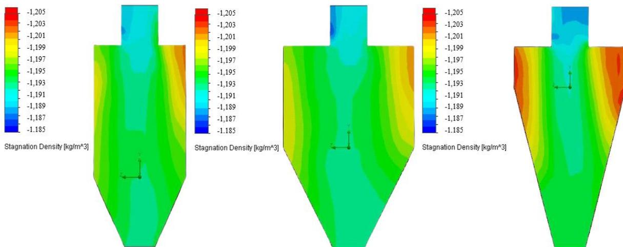
Figure 6. Longitudinal section of cyclones No. 1-3 showing the internal distribution of the density of air, polluted with lignite dust, with a forced volumetric flow of  $0.7 \text{ m}^3/\text{s}$ .
