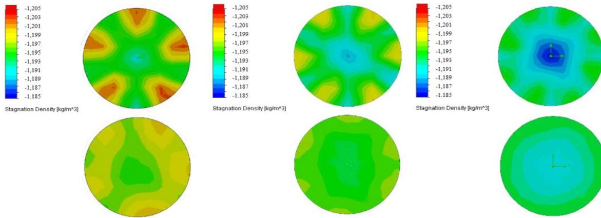
Figure 11. Longitudinal section of a MOS cell (cyclones No. 1 in the left figure, No. 2 in the centered figure, No. 3 in the right figure), equipped with 5 blades (left figure), 6 blades (centered figure) and 8 blades (right figure) inclined at an angle of 45°, showing the distribution of the density of the air, behind the blades and polluted with lignite dust (top row picture), and at the outlet (bottom row picture) with a volumetric flow of 0.4 m<sup>3</sup>/s.
