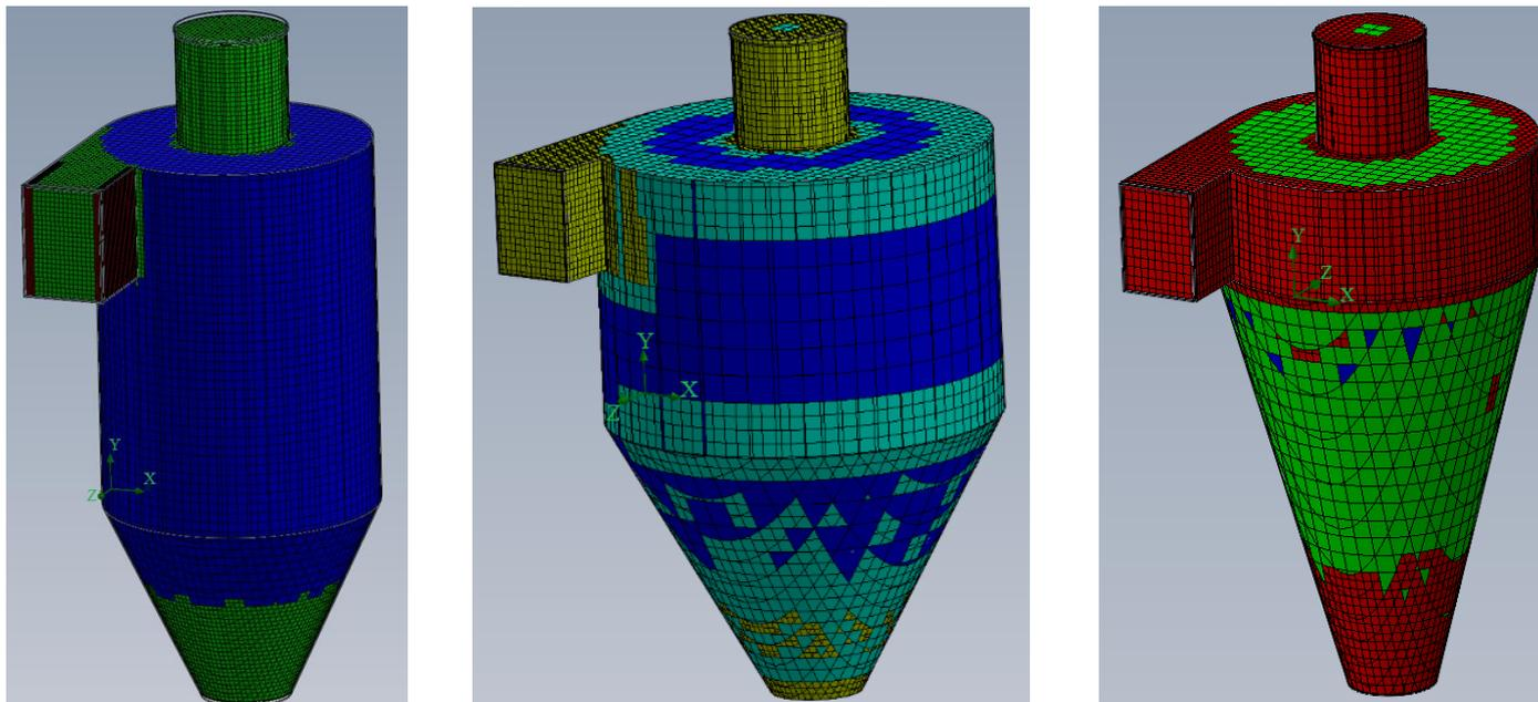
Figure 4. Computer models of designed cyclones: Cyclone No. 1 with a body height of 750 mm, a 250 mm hopper and a corpse diameter of 250 mm in the left photography; Cyclone No. 2 with a body height of 500 mm, a discharge hopper of 500 mm and a corpse diameter of 350 mm in the centered photography; Cyclone No. 3 with a body height of 150 mm, a discharge hopper of 850 mm and a hull diameter of 300 mm in the right photography ( $x, y, z$  – parameters of the Cartesian system).
