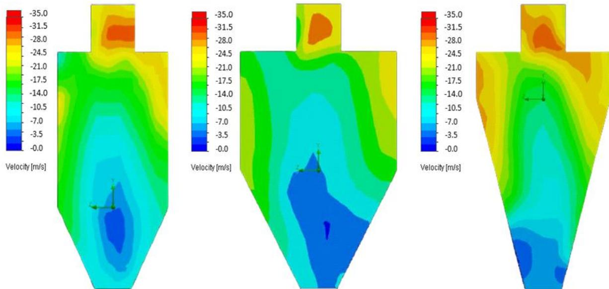
Figure 5. Longitudinal section of cyclones No. 1 in the left figure, No. 2 in the centered figure, No. 3 in the right figure, showing the internal velocity distribution of air, polluted with lignite dust, with a forced volumetric flow of  $0.7 \text{ m}^3/\text{s}$ .
