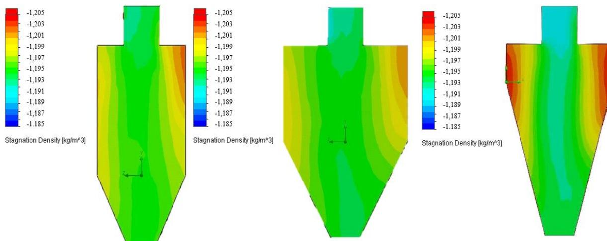
Figure 8. Longitudinal section of cyclones No. 1 in the left figure, No. 2 in the centered figure, No. 3 in the right figure, showing the internal distribution of the density of air, polluted with lignite dust, at a volume flow of 0.5 m<sup>3</sup>/s.
