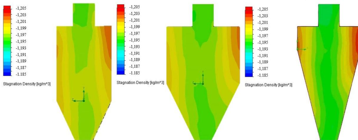
Figure 7. Longitudinal section of cyclones No. 1 in the left figure, No. 2 in the centered figure, No. 3 in the right figure, showing the internal distribution of the density of air, polluted with lignite dust, at a volume flow of 0.3 m<sup>3</sup>/s.
