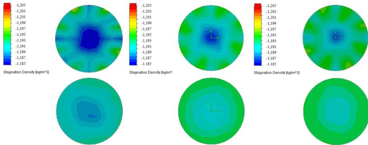
Figure 13. Longitudinal section of a MOS cell (cyclones No. 1 in the left figure, No. 2 in the centered figure, No. 3 in the right figure), equipped with 8 blades, inclined at an angle of 30° (left figure), 45° (centered figure) and 60° (right figure) showing the distribution of the density of the air, behind the blades, polluted with lignite dust (top row picture), and at the outlet (bottom row picture) with a volumetric flow of 0.4 m<sup>3</sup>/s.
