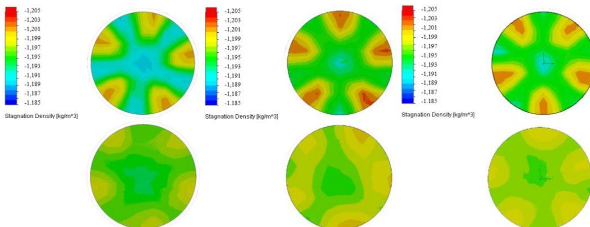
Figure 12. Longitudinal section of a MOS cell (cyclones No. 1 in the left figure, No. 2 in the centered figure, No. 3 in the right figure), equipped with 5 blades inclined at an angle of 30° (left figure), 45° (centered figure) and 60° (right figure) showing the distribution of the density of the air, behind the blades and polluted with lignite dust (top row pictures), and at the outlet (bottom row pictures) with a volumetric flow of 0.4 m<sup>3</sup>/s.
